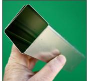
**Test**: A three-axis sensor was used at the centre of the shields. The local Earth's field was used as magnetic field, to which a 50 Hz component was added. The X-axis of the sensor was placed in North-South direction. The Z-axis is vertical. These magnetic measurements were made with an instrument Bartington Spectramag-6, with a probe Mag-03MS1000.
