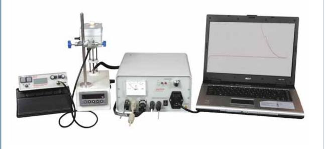
This system is used in the investigation of magnetic mineralogy and grain size and for the determination of Curie transition temperatures. It permits magnetic susceptibility measurements to be made on 15mm diameter (2.5ml) samples over the temperature range  $-200^{\circ}$ C to  $+850^{\circ}$ C.
