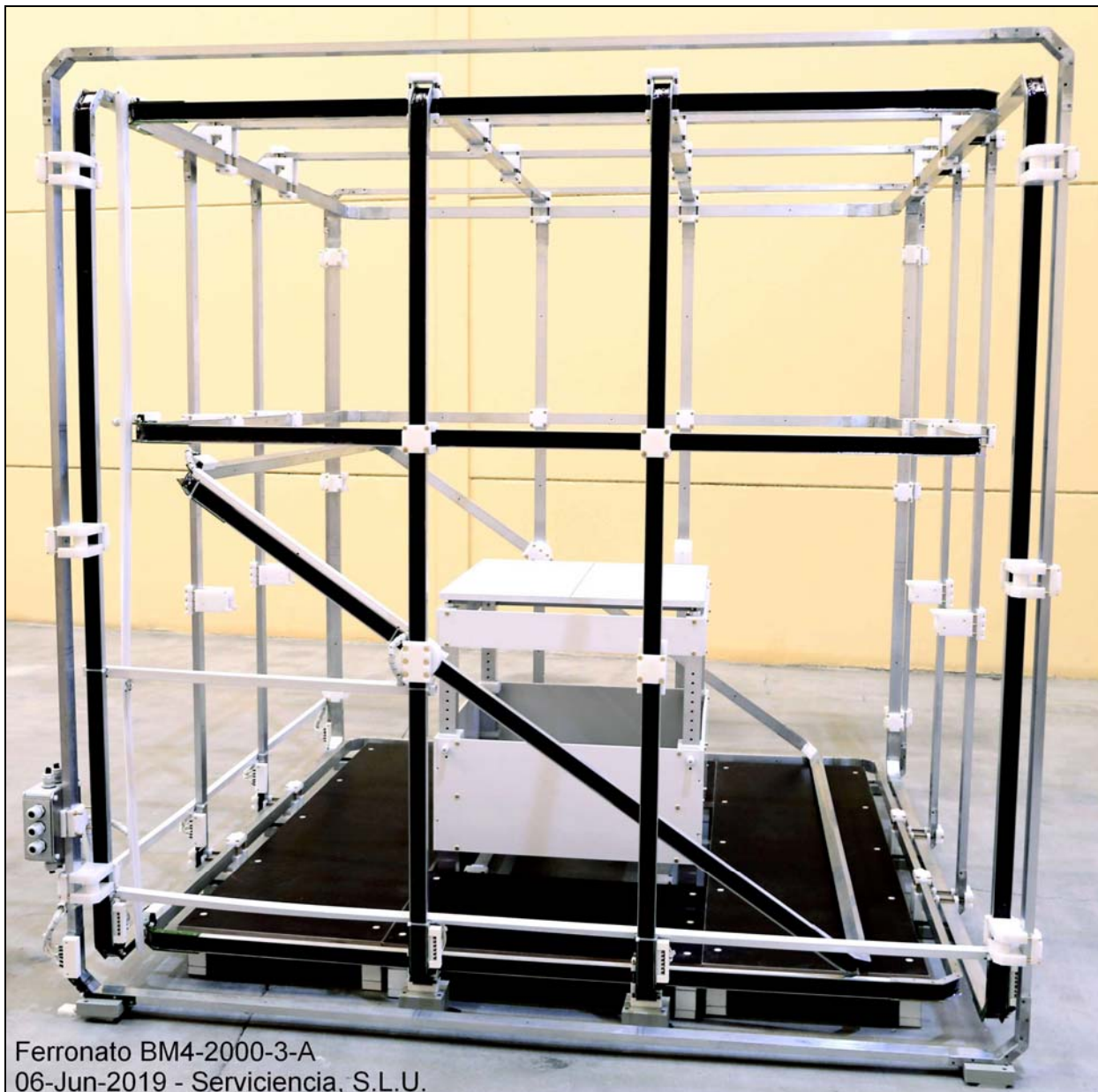
Fig. 1: A photo of the system, with optional DUT stand and elevated floor.
